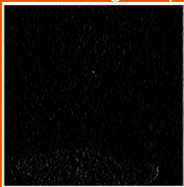
Vertical edges of potholes
